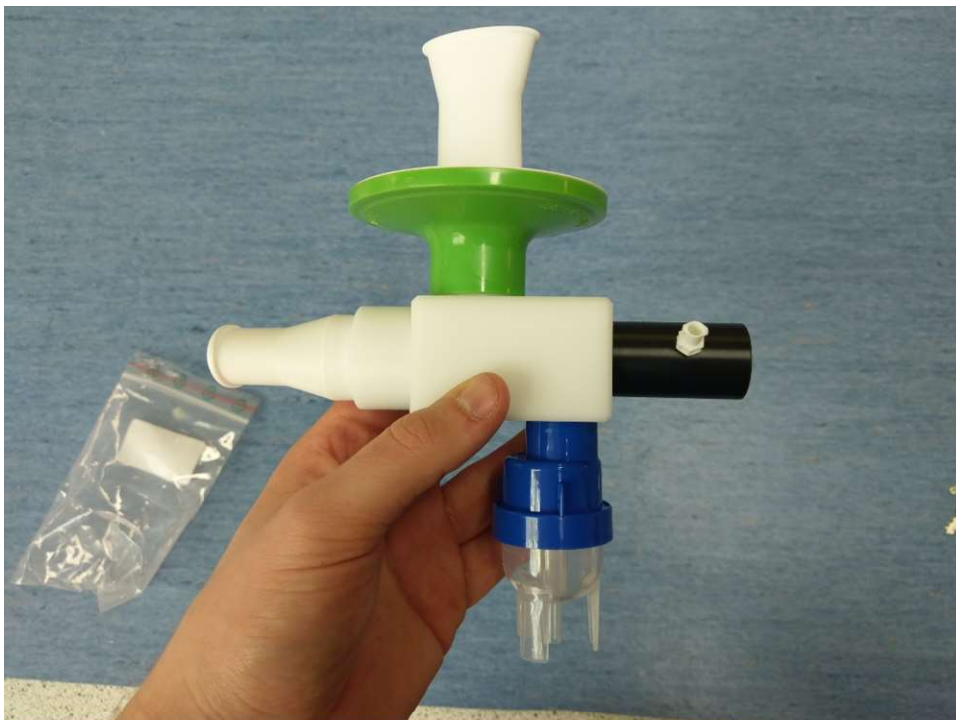
Figure 1 Completely assembled nebulizer valve without tubes connected
